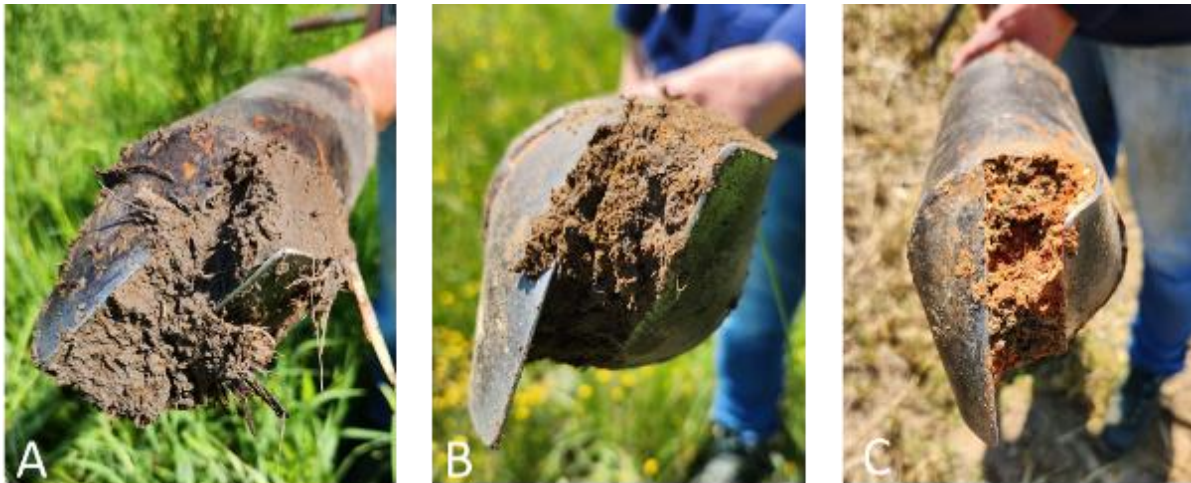
Figure 7-9: Hydric soils identified in the wetland systems including the (A) Katspruit, (B) Pinedene and (C) Bloemdal soil forms
