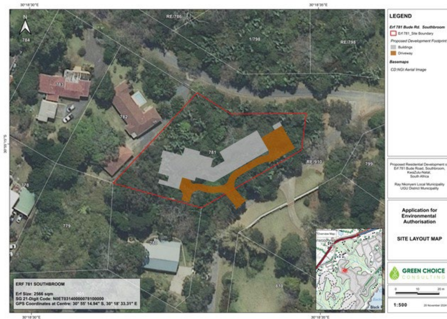
Satellite image showing the project property outlined in red, with the shaded areas depicting the proposed development footprint.
