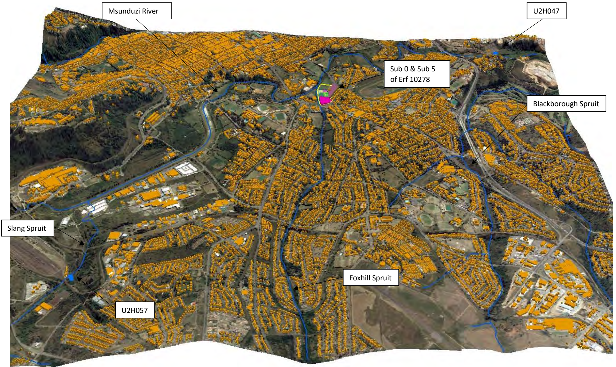
Figure 10 Exaggerated (x3) Digital Elevation Model (DEM) of the catchment surrounding Woodburn Shopping Centre
