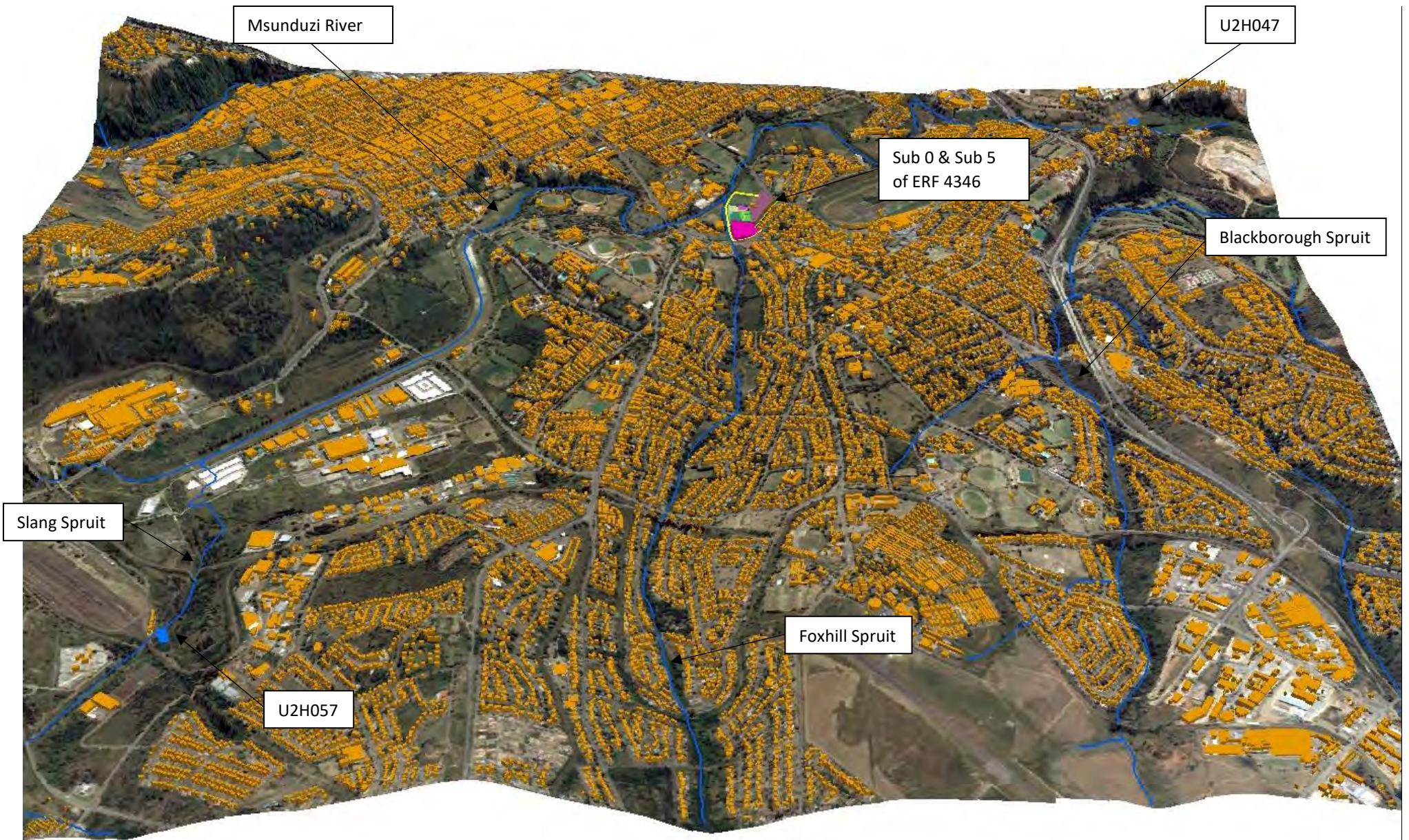
Figure 8 Exaggerated (x3) Digital Elevation Model (DEM) of the catchment surrounding Woodburn Shopping Centre
